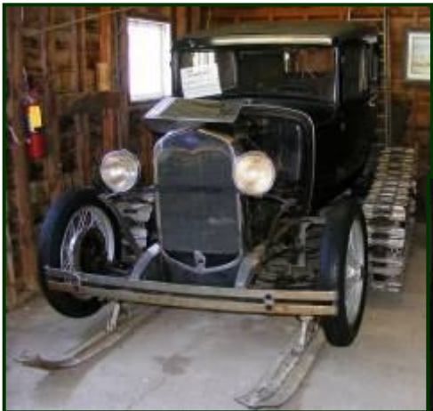
1930 MODEL A SNOWMOBILE "SNO-BIRD" CONVERSION KIT MADE IN NEW HOLSTEIN, WISC. OWNED BY WASHINGTON ISLAND MUSEUM USED TO HAUL SUPPLIES TO ISLANDS OVER ICE
